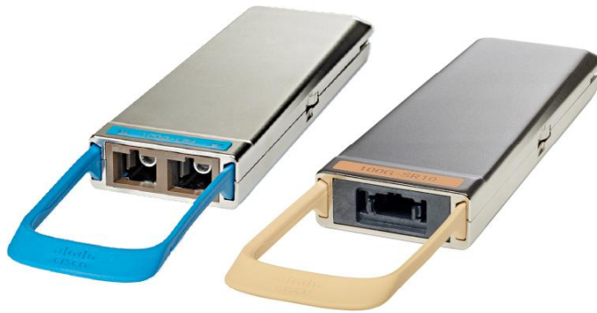
Figure 2. Cisco CPAK 100GBASE-LR4 Module (left) 100GBASE-SR10 Module (right)
