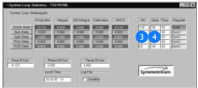
Gears 1, 2, and 3 are warm-up processes after power-up. Gears 4, 5, and 6 indicate a settling period when the TimeSource 2700 outputs Stratum 1 signals. Gear 7 indicates steady-state operation.
